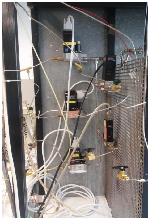
Figure B-1: Mass flow controllers to provide a flow of the components
